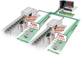
module can directly count out the frequency in site. This reduces the frequency errors caused by communication latency between two ends, and also reduces the network loadings. In order to applying for more applications, this module provides 3 scan modes (0.1s, 1s and single-pulse) and 4 moving average levels for user to select the best way in their applications. This feature can be used for rotation and speed measurements... etc.
