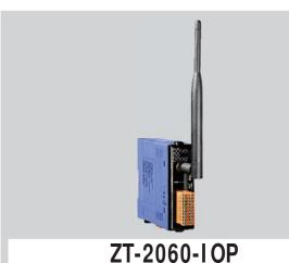
ZigBee I/O Pair-connection Module with the 4-channel Isolated Digital Input and 4-channel Relay Output
